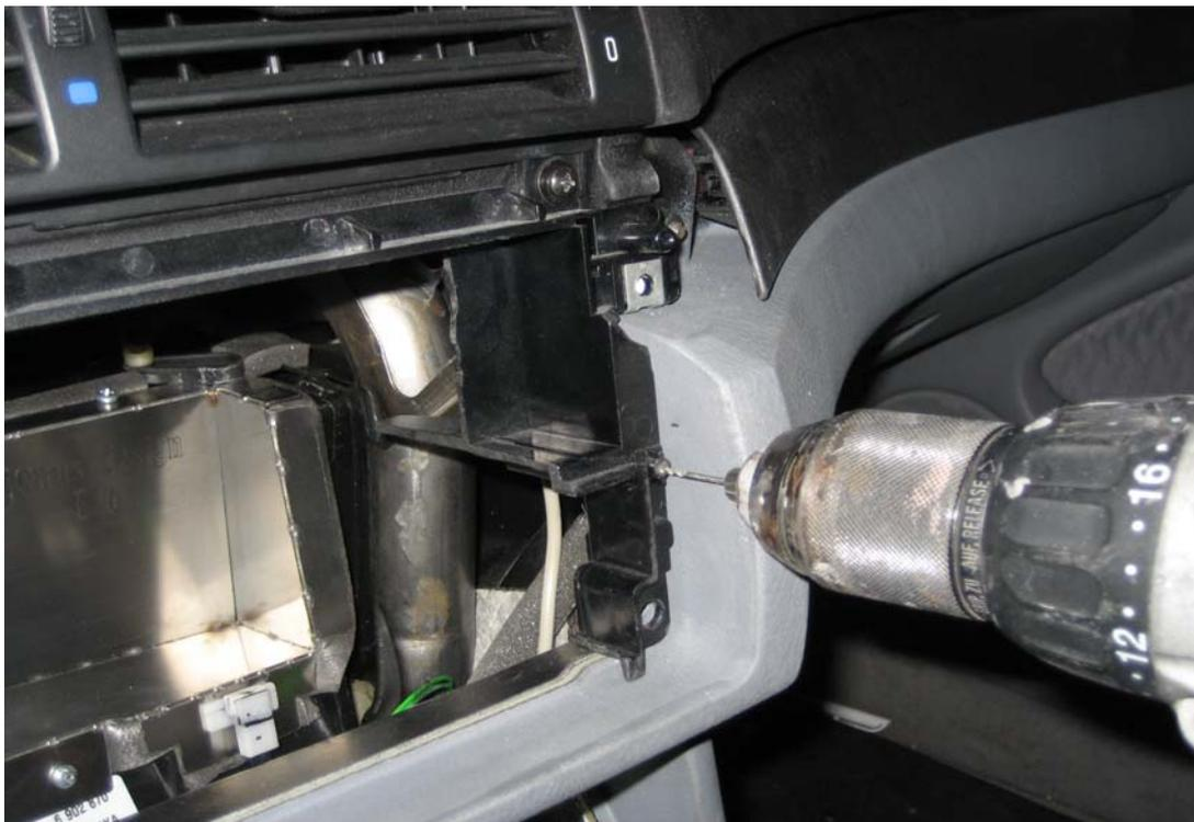
Replace the radio holder and now drill 2mm holes through the cutted bolts through the dashboard (long drill)
