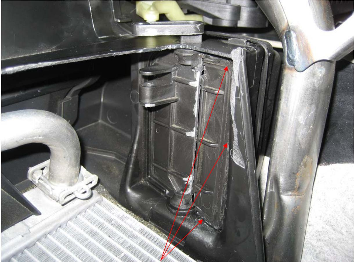
Replace the flap again with the big screw driver, glue the cutted front-part with super-glue at the case. Clean the both gluing-sides with thinner and sand it locally, cause BEHR used vaseline for better flap movement
