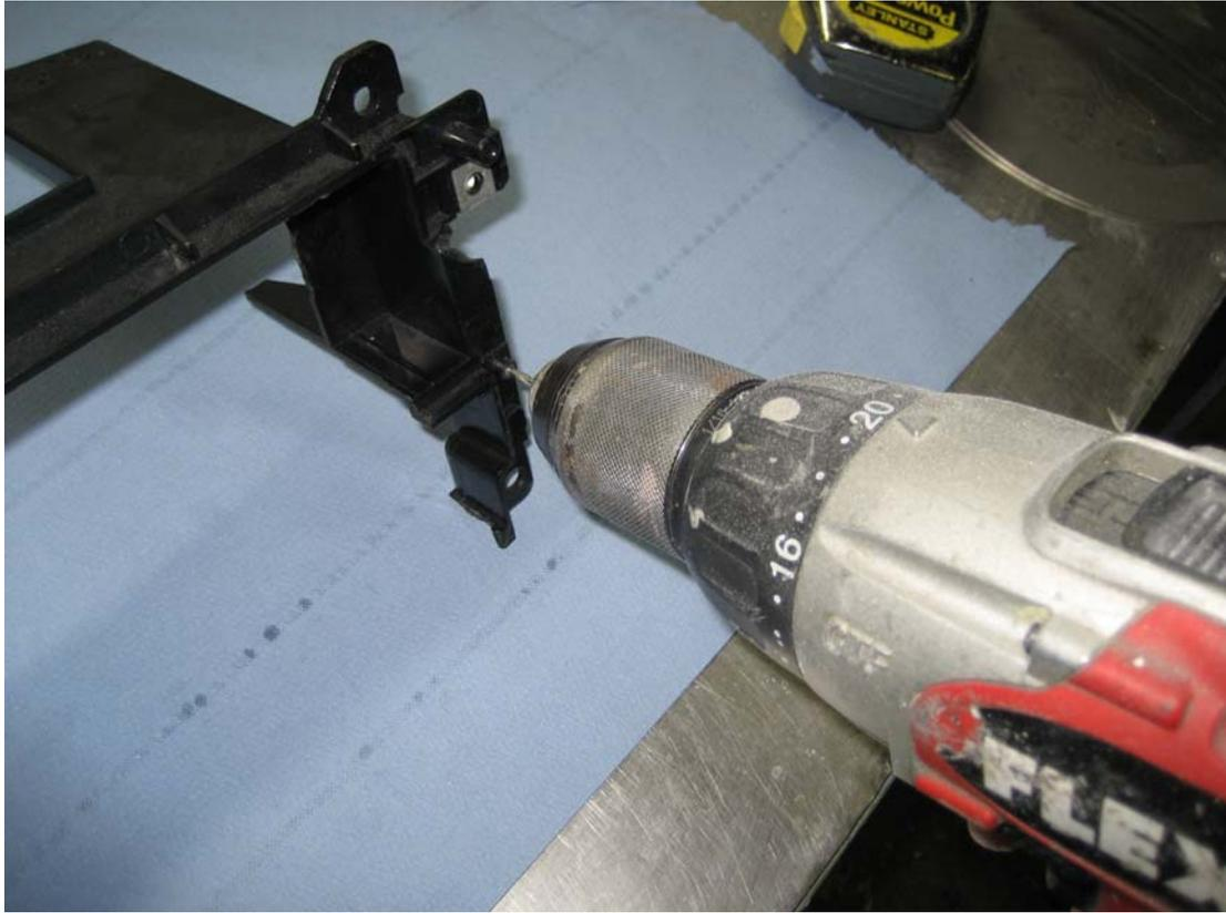
Drill 2mm holes through the planed bolts on both sides
